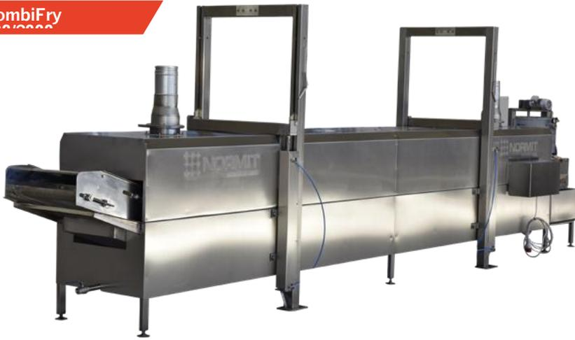
**CombiFry 500/2000** – with the combination of immersion frying. The high oil turnover, its intensive circulation and constant filtration, ensure a superior quality of the final product and the preserving its nutritional properties. The method of pouring hot oil is an ideal solution for frying meat, fish, vegetables, dough products, snacks (hard and fragile structure), both breaded and non-breaded.
